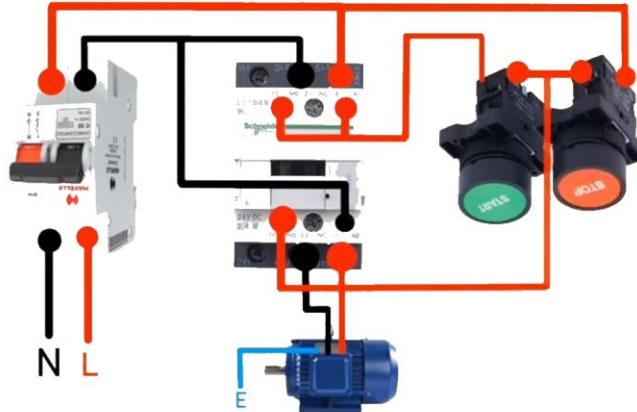
Single phase motor connection with magnetic contactor
