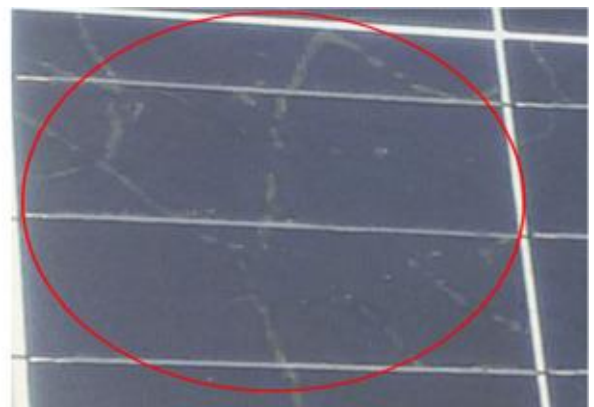
b. Delamination of encapsulant of 8-year old polycrystalline module in Wet Semi Equatorial Climatic Zone
