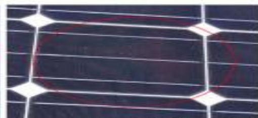
j. Slightly brown discoloration of encapsulant of 5-year old monocrystalline module in Dry Equatorial Climatic Zone
