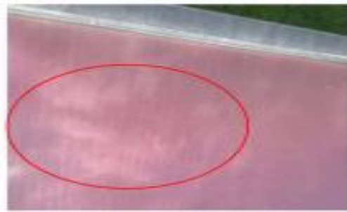
b. Light discoloration of encapsulant of 10-year old amorphous module in Dry Equatorial Climatic Zone
