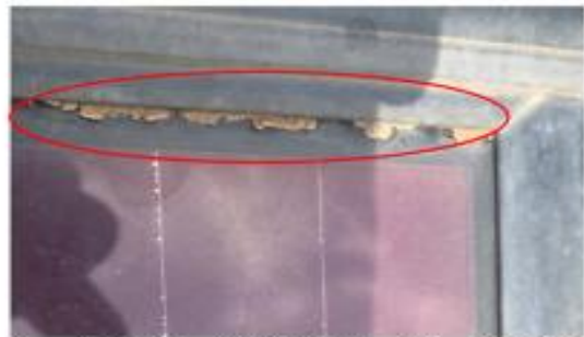
b. Sealant infiltration of 10-year old amorphous silicon module in Dry Equatorial Climatic Zone
