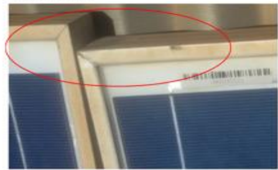
f. Minor corrosion on frame of 8-year old polycrystalline module in Wet Semi Equatorial Climatic Zone
