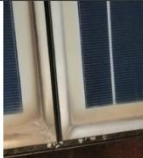
(3a) Dark discoloration of encapsulant, minor corrosion of frames
