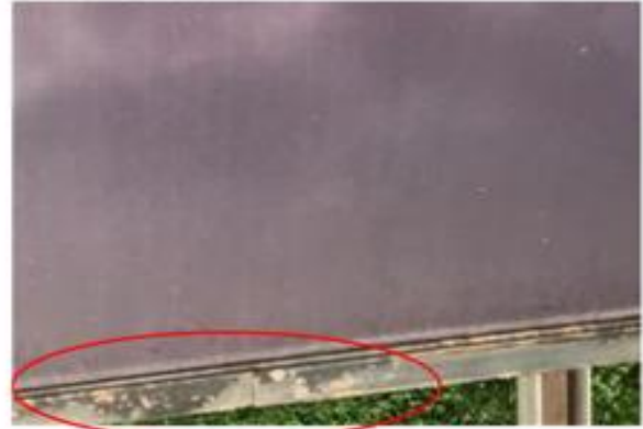
b. Sealant infiltration of 10-year old amorphous silicon module in Dry Equatorial Climatic Zone
