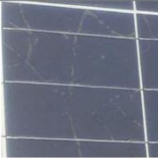
(4a) Delamination of encapsulant, minor corrosion of frame
