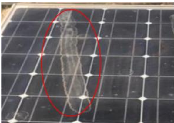
a. Delamination of encapsulant of 15-year old monocrystalline module in Tropical Continental or Interior Savannah Climatic Zone
