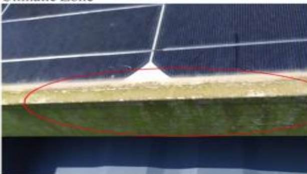
g. Minor corrosion on frame of 5-year old monocrystalline module in Dry Equatorial Climatic Zone
