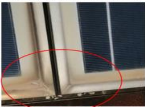
e. Minor corrosion on frame of 8-year old polycrystalline module in Wet Semi Equatorial Climatic Zone
