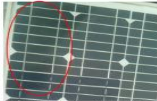
d. Slightly yellow discoloration of encapsulant of 15-year old monocrystalline module in Tropical Continental or Interior Savannah Climatic Zone
