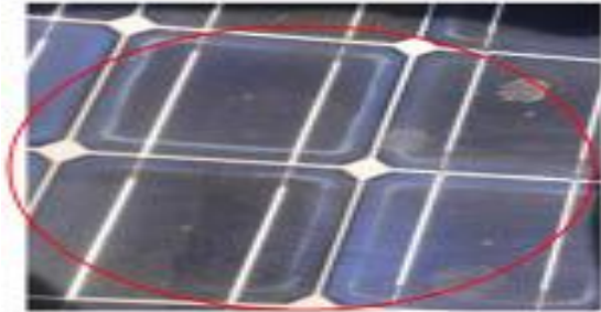
c. Light blue discoloration of encapsulant of 15-year old monocrystalline module in Tropical Continental or Interior Savannah Climatic Zone
