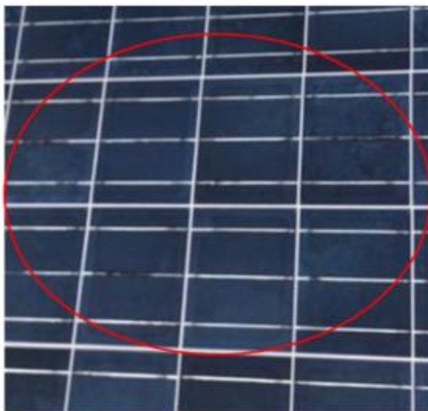
c. Minor discoloration of metallisation of 8-year old polycrystalline module in Wet Semi Equatorial Climatic Zone
