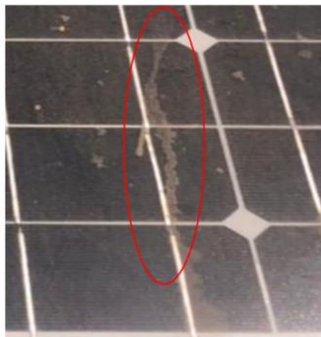
b. Minor crack on 15-year old monocrystalline module in Tropical Continental or Interior Savannah Climatic Zone
