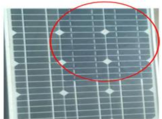
b. Light discoloration of metallisation of 15-year old monocrystalline module in Tropical Continental or Interior Savannah Climatic Zone
