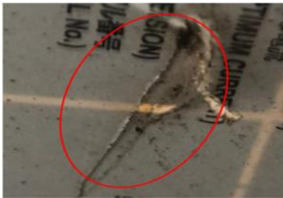
a. Backsheet scratch of 8-year old polycrystalline module in Wet Semi Equatorial Climatic Zone
