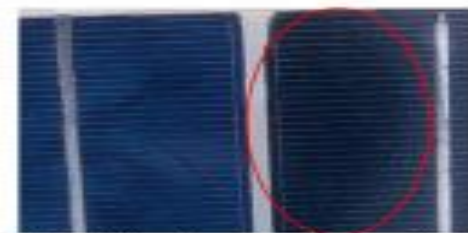
h. Dark discoloration of encapsulant of 8-year old polycrystalline module in Wet Semi Equatorial Climatic Zone
