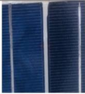
(3a) Dark discoloration of encapsulant, minor corrosion of frames
