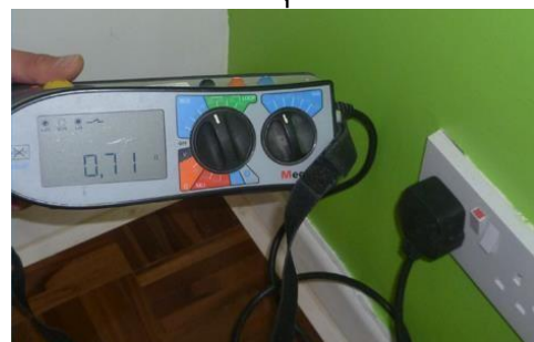
Earth Loop Impedance Test of Z_s at Socket Outlet
